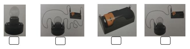
Step \_\_\_\_\_: Open the clamps and connect one of the wires to one end of the battery holder and one side of the bulb holder.
